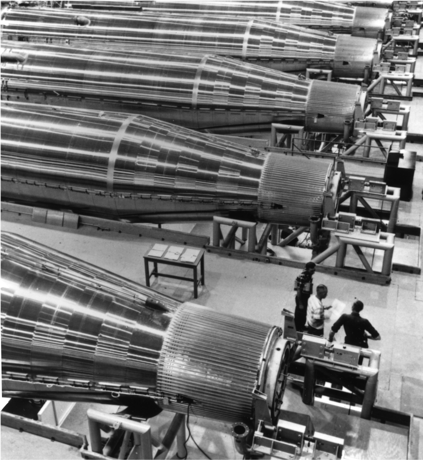
Atlas missiles on the production line at the San Diego, California, plant of General Dynamics Corporation's Convair Division in 1958. Unlike aircraft, which required only a few test vehicles, missiles required an assembly line right from the outset.
