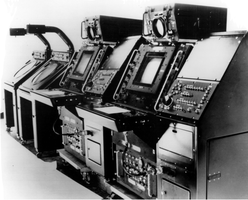
SAGE equipment in 1958 included video mappers, radar height indicators, and antenna control units.
