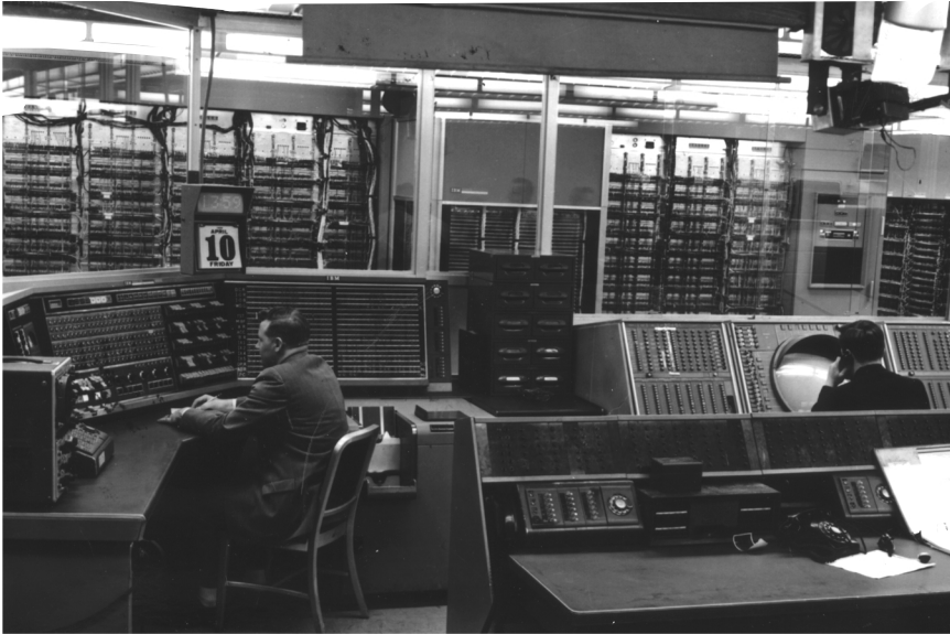
Control consoles of the XD-1 computer for SAGE experimentation. Originally, the XD-1 was known as Whirlwind II, but it was renamed by the Lincoln-IBM team.
