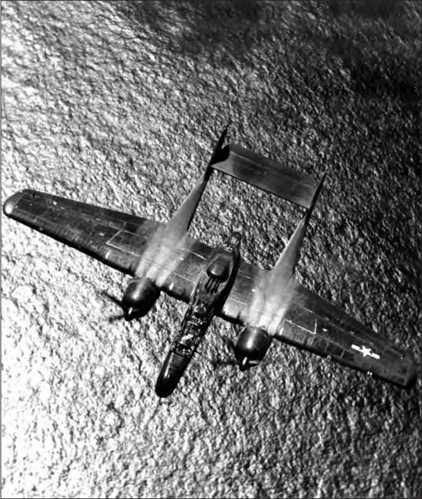
A P-61 from the top. The three crew positions, from front to back, are the pilot, gunner, and radar operator.
