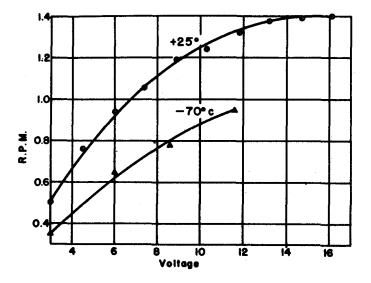
Figure 32. Speed tests of Olland-Cycle motors.
