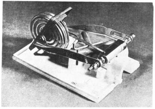
Figure 11. Pressure displacement switch.
