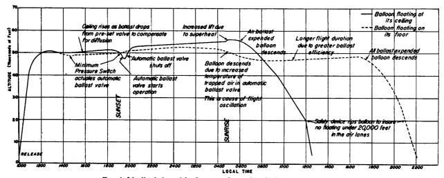
FIG. 6. Idealized time-altitude curves for various balloon-control systems.
