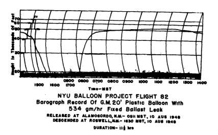
Fig. 8 Balloon Flight Using Fixed Ballast Flow
