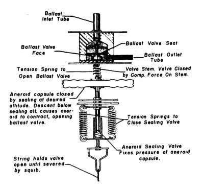
Figure 10. Automatic ballast valve.
