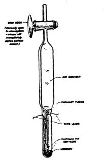
FIG. 4. Minimum pressure switch (mercurial).
