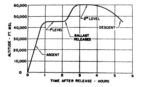
Fig. 15 "Two Level" Stepped Flight
