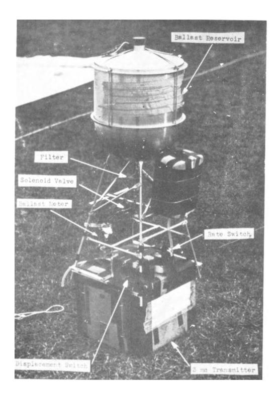
Figure 10 Ballast reservoir assembly showing component parts
