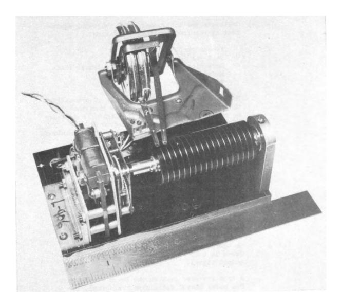
Figure 31 Olland Cycle Pressure Modulator gears or poor alignment of the rotating cylinder. The motor gears may be cleaned with carbon tetrachloride and a small clean brush. If the trouble is due to misalignment, the instrument should not be used since this will affect the rotation at a non-uniform rate and thus destroy the entire accuracy of the record.
