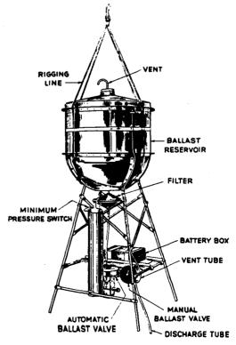
FIG. 3. Ballast-release assembly.
