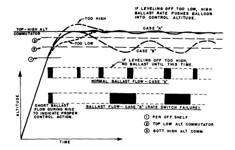
Figure 15. Theoretical height-time curve.
