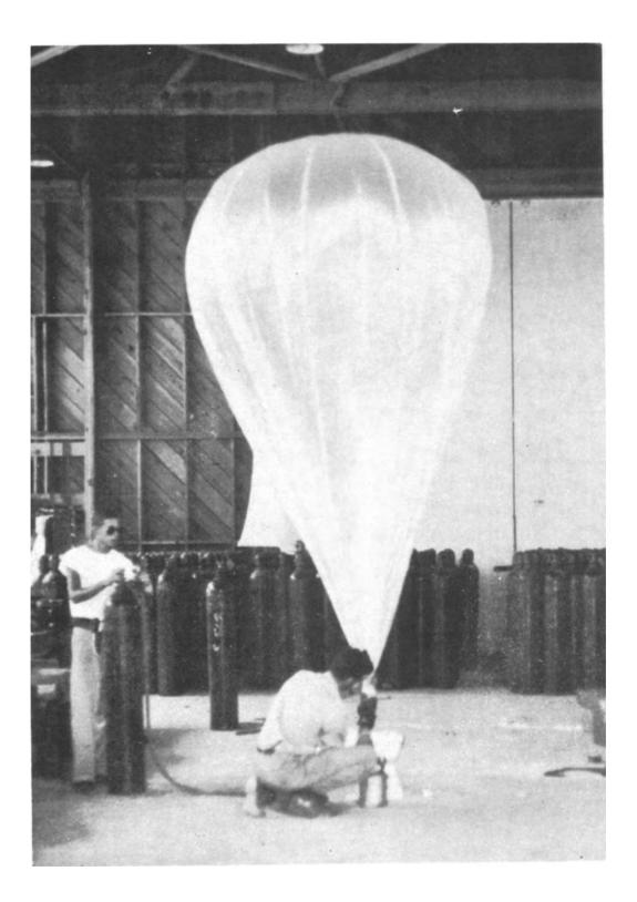
Figure 40 General Mills 7 foot balloon being inflated. of 170 grams per hour. A balloon of this type with no altitude control stayed aloft for more than two hours and after reaching ceiling, the altitude did not vary by more than 1500 feet while the balloon was within range of the ebserving station.
