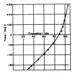
Figure 34. Sample celibration chart for temperature measurements.
