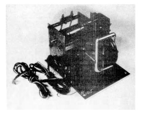
Fig. 1 Pressure Displacement Switch for Ballast Control
