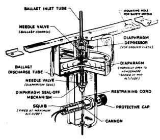
FIG. 2. Automatic ballast valve.
