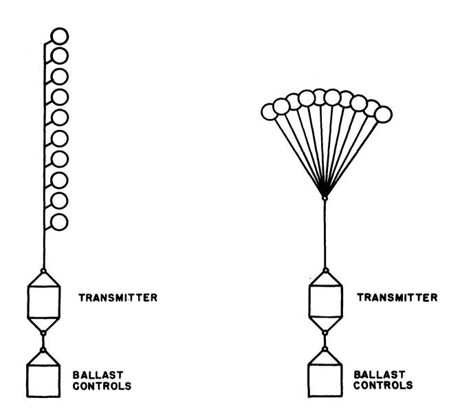
Figures 3 and 4. Typical rubber balloon arrays.
