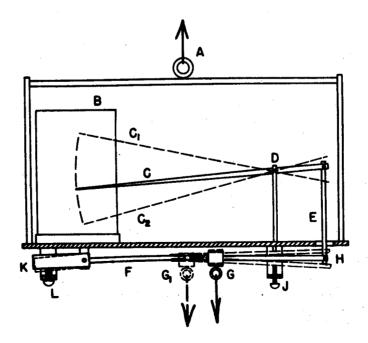
Figure 38. Ballast-recording meter.
