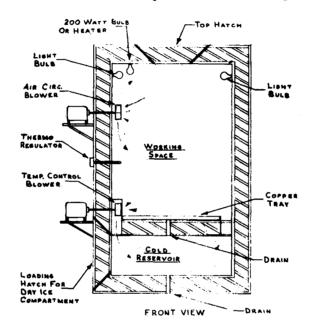
LOWEST WORKING TEMP -65" To-70" C ACCURACY OF TEMP CONTROL 0.5"C
