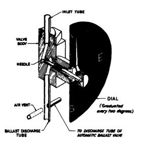
Figure 9. Manual ballast valve.
