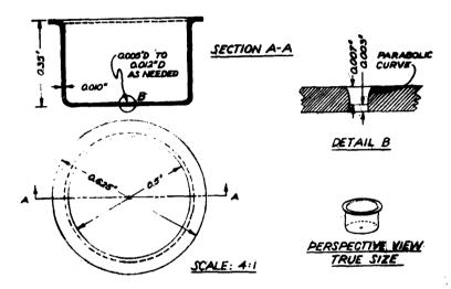
Figure 8. Orifice for fixed-rate ballast flow.
