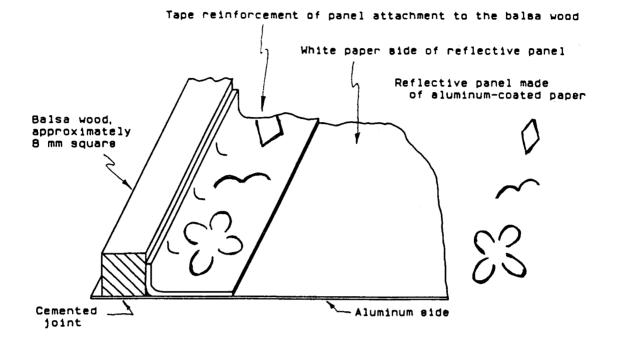
MY RECOLLECTION OF THE REFLECTOR MATERIAL ATTACHMENT TO THE BALSA WOOD PIECES ON THE ML-307/AP PILOT BALLOON RADAR TARGETS IN 1947.
