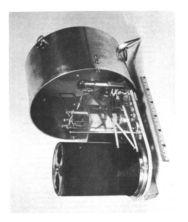
temperature recording is confined to the lower 2 inches of the drum so as to interfere as little as possible with the pressure record when the balloon floats above 30,000 feet.
