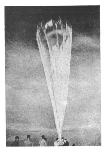
Figure 5. 20'-Diameter, teardrop polyethylene balloon. In all of these, film is .001" polyethylene, butt welded with fiber tape laid along the seams to reinforce the seal, and to carry and distribute the load. These tapes, which converge to the load ring at the bottom, actually support the load (Figure 6). An open bottom permits the escape of excess lifting gas and thus prevents rupture.
