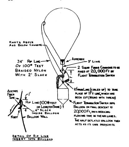
Figure 21. Flight termination equipment.
