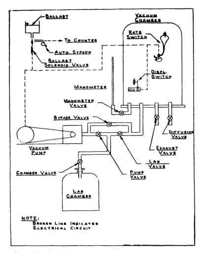
Figure 20. Physical layout, flight-similitude system.
