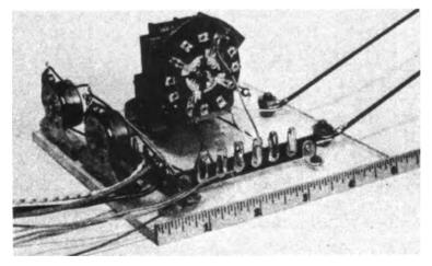
Figure 36. Temperature programming switch.
