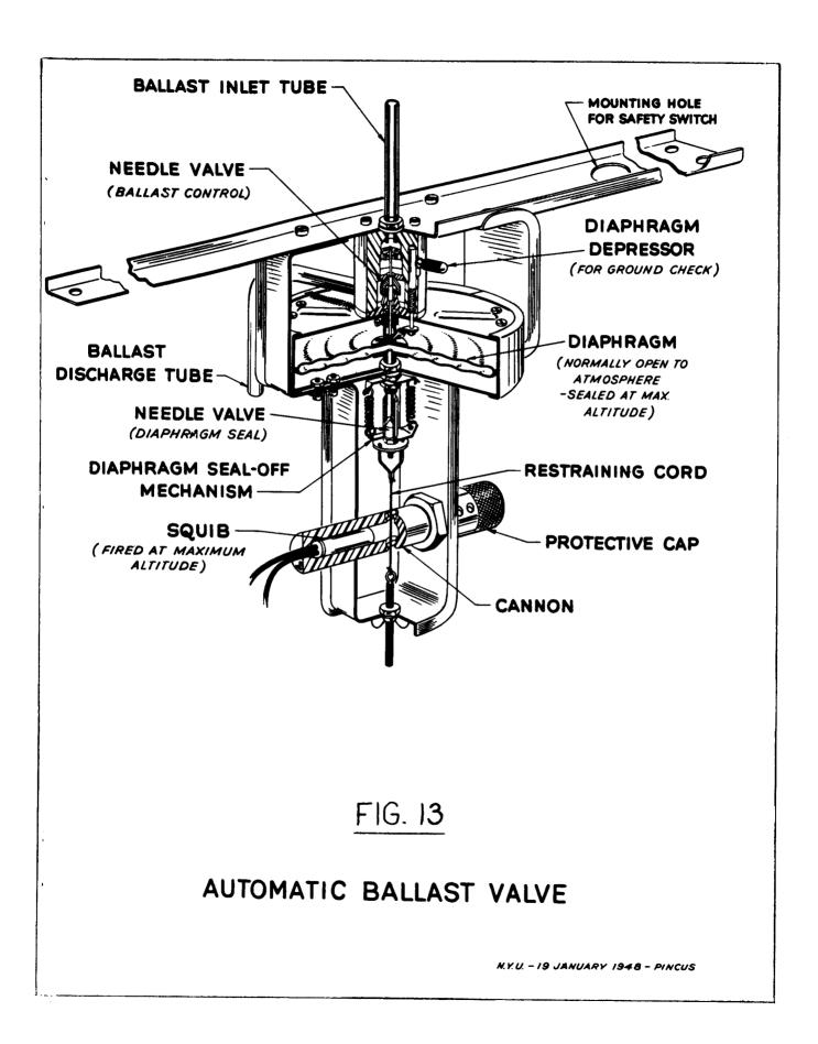
When the atmospheric pressure outside the diaphragm increases to 5 mb. above the internal pressure, compass fluid will be discharged at the rate of 160 grams per minute under a 1-foot head. When the automatic ballast valve is completely open (at 6.5 mb. pressure differential), 300 grams per minute will flow.
