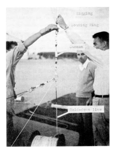
Figure 27 Aluminum "cannon" and launching lines used to restrain balloon while load is being attached. the total strain on rigging lines and even on the balloon itself becomes excessive. With the thin polyethylene film of the General Mills' balloons, such a wind force causes the balloon first to billow, sail-like, as in Figure 25, then to tear.
