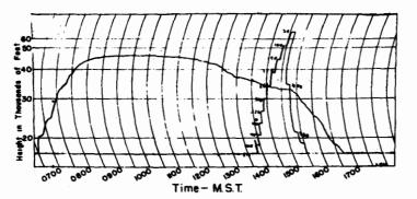
NYU BALLOON PROJECT FLIGHT 70 Showing 20' General Mills Balloon Performance When No Ballast Was Dropped RELEASED AT HOLLOMAN AFB, NM-JULY 8, 1948 0633 MST - RECOVERED AT KENT, TEXAS Figure 25
