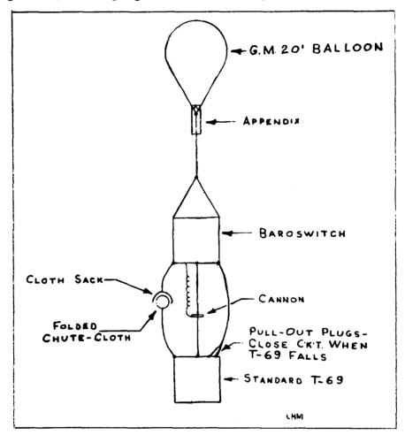
Figure 36: Equipment train, Flight 85
