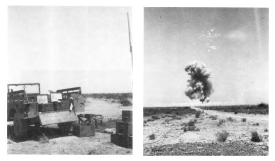
Sitting in the back of the truck (*left*) is a U.S. Army GR-3 Sound Ranging Set, normally used by field artillery observation units but adapted for use in Project MOGUL. The set was employed for the MOGUL operations at White Sands Proving Ground in July 1947. The detonation, or "shot" (*right*), of 500 pounds of TNT was monitored at White Sands Proving Ground, NM, in July 1947, by Project MOGUL balloon and ground-based sensors. *Photo Collection of Albert P. Crary.*
