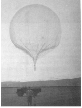
This 15-foot polyethylene balloon (*left*) and 70-foot polyethylene balloon (*above*) are representative of the type used extensively by Project MOGUL. It is this variety of balloon that caused many UFO sightings due to their flat, spherical appearance when viewed from the ground.
