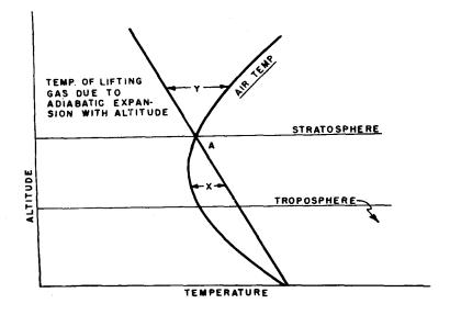
Figure 22. Lapse rate of air and helium.
