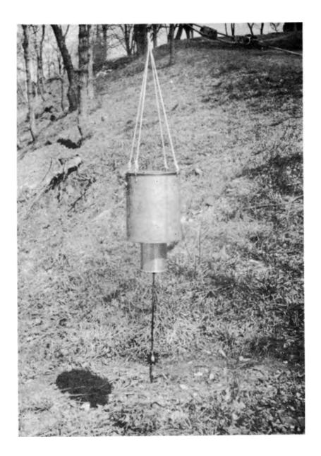
Figure 9 Fixed rate, manually operated ballast release assembly.
