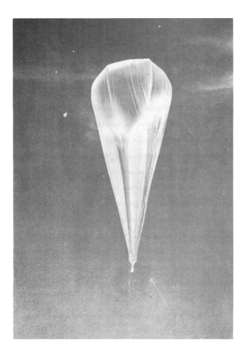
Figure 6 General Mills 20 foot balloon in flight with 2 foot stiffened appendix. various cluster arrangements. None of these have been too satisfactory but further investigation will be made in the field of shrouded or coated films.
