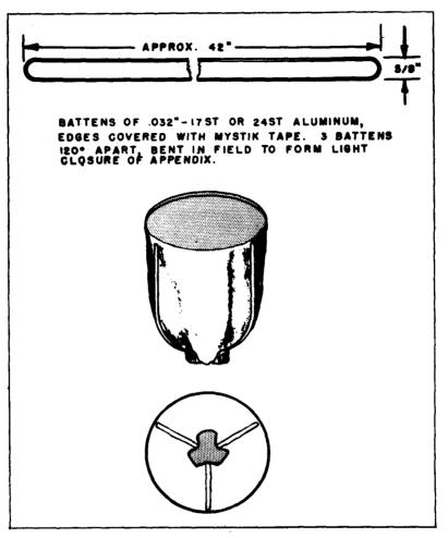
Figure 30: Aluminum battens for balloon appendix
