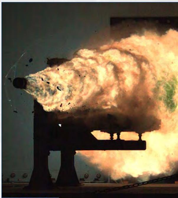
This photograph was taken from a high-speed video camera during a record-setting firing of an electromagnetic railgun (EMRG) at Naval Surface Warfare Center, Dahlgren, Virginia. U.S. Navy Photograph.
