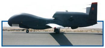
A Global Hawk unmanned system vehicle is towed back to its hangar following a mission at a deployed location in Southwest Asia. Once mission parameters are programmed into a Global Hawk, the UAS can autonomously taxi, take off, fly, remain on station capturing imagery, return and land. Ground-based operators monitor the UAS's status, and can change navigation and sensor plans during flight as necessary.
