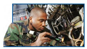
Airman 1st Class Marlon Wells uses a flashlight to visually inspect the avionics system in the cargo bay of a C-130 Hercules aircraft.
