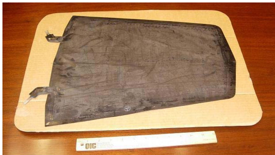
Figure 1. C-130 Aircraft Propeller Blade Heater Manufactured by SMR
