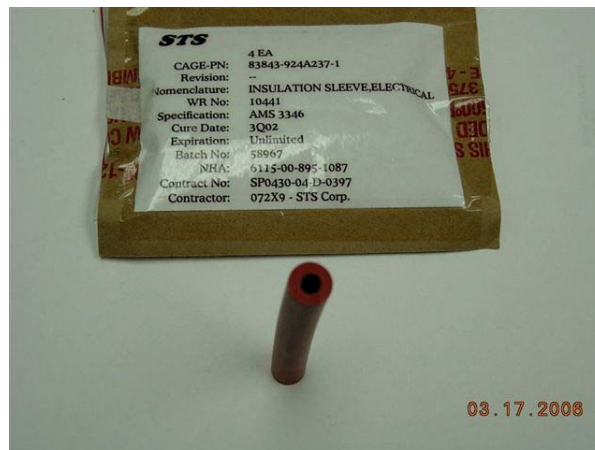
Figure 4. Insulation Sleeve for the T-38 Aircraft Supplied by Hamilton Sundstrand
