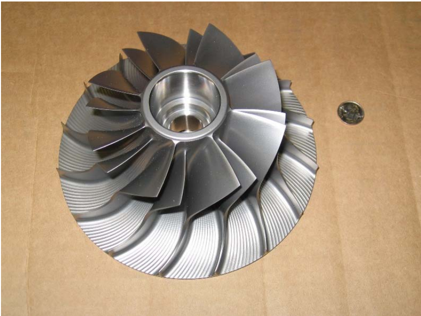
Figure 10. Compressor Wheel Supplied by Hamilton Sundstrand
