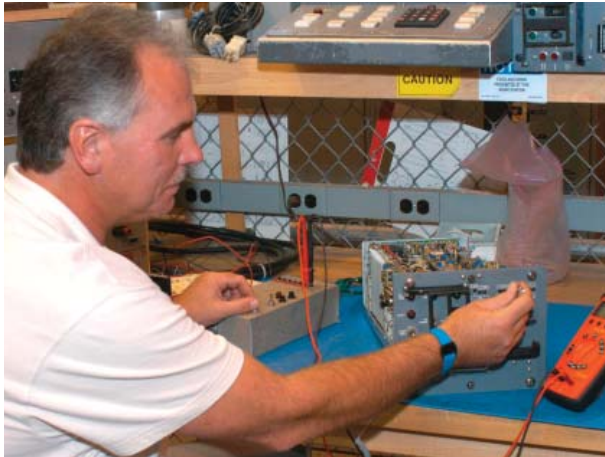
Bruce Telincho, a Pittston Township resident, tests a telephone circuit switch power supply component at Tobyhanna Army Depot. The component will be used in AN/TTC-46 and 47 Mobile Subscriber Equipment. (by Anthony Ricchiazzi)
