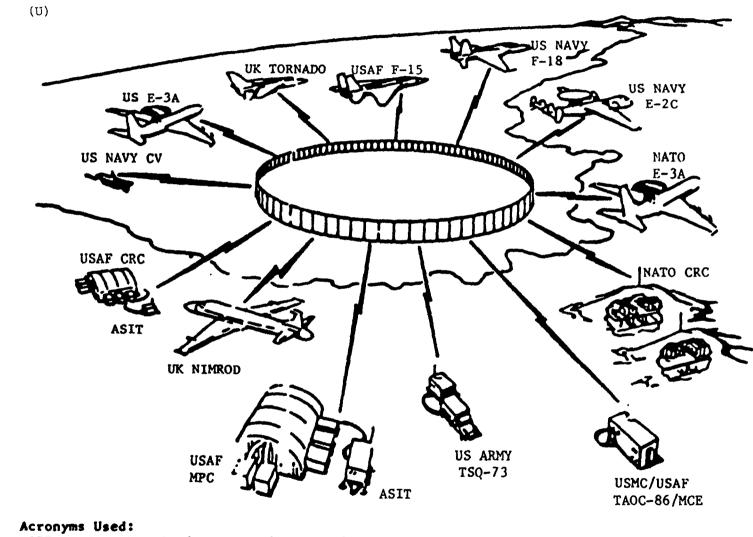
ACTONYMS Used: ASIT - Adaptable Surface Interface Terminal CRC - Control and Reporting Center CV - Carrier Unit MPC - Message Processing Center TAOC/MCE - Tactical Air Operations Center; Mobile Control Equipment TSQ - Transportable Special Equipment
