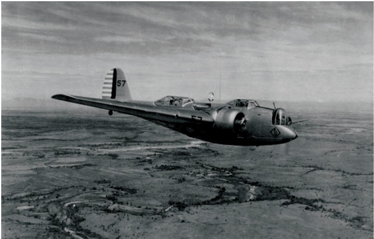
The Martin B-10 was the fastest and most heavily armed bomber at the time (1934). It had a gross weight of 14,731 pounds, a 4-man crew, and was powered with 2 Wright 740 horsepower engines capable of a top speed of 212 miles per hour.
