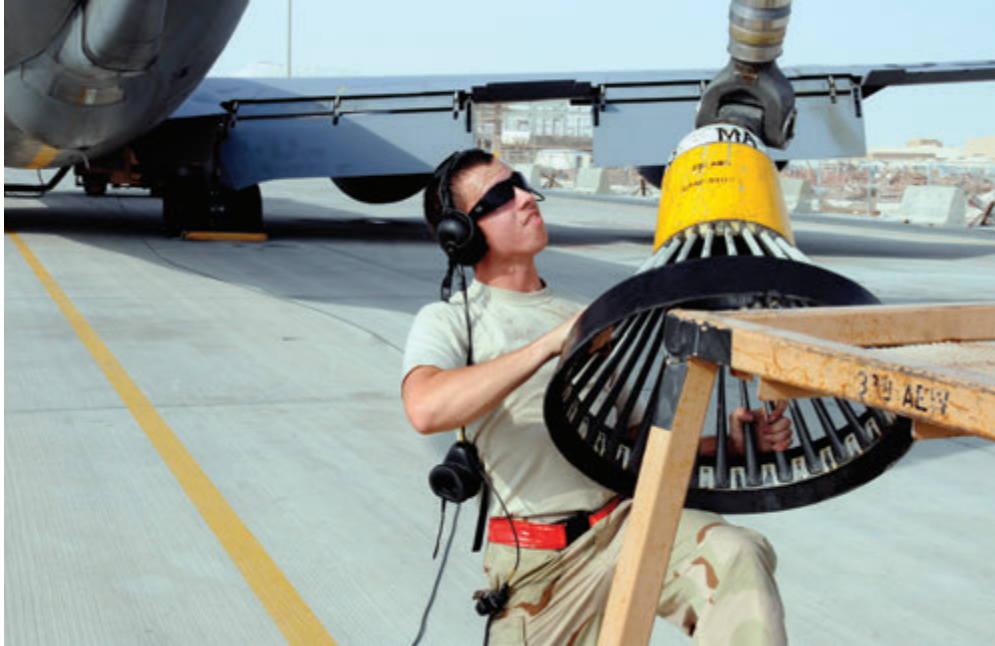
As part of the preflight checklist, Airman 1st Class Jason Somrak, serving with the 379th Expeditionary Aircraft Maintenance Squadron, muscles the KC-135 Stratotanker aircraft refueling pod off of the stand on the flightline of an undisclosed airfield in Southwest Asia, 10 September 2008. (US Air Force photo by TSgt Michael Boquette)
