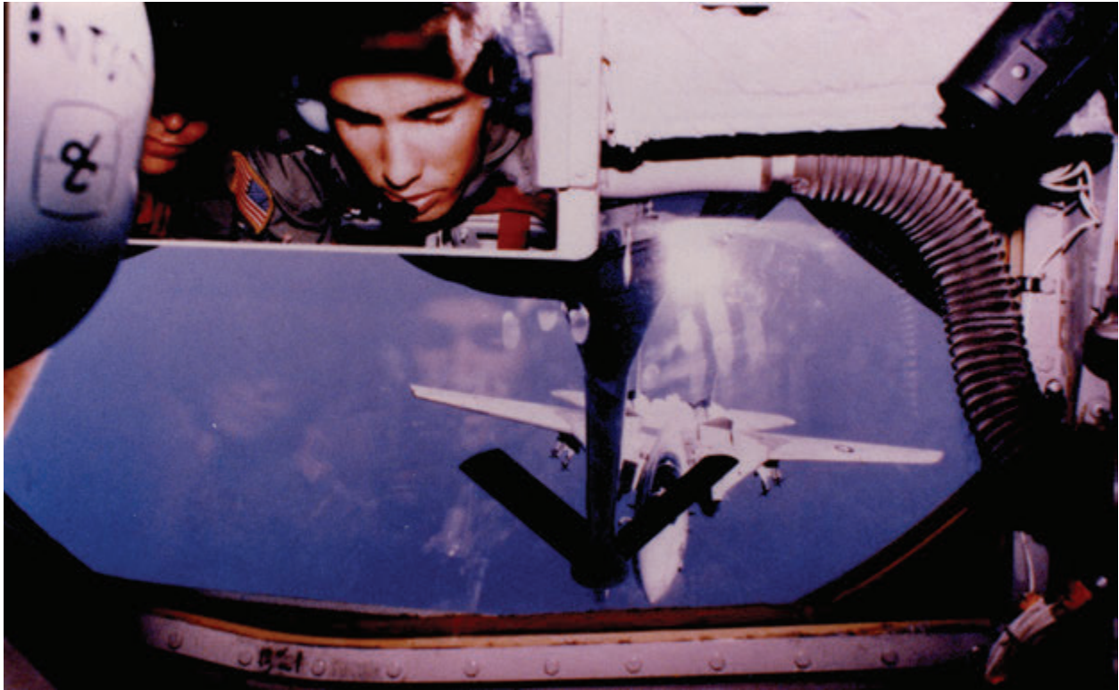
A boom operator on a KC-135 uses a boom-drogue adapter to refuel a US Navy F-14 Tomcat.
