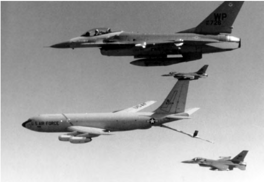
The KC-135 Stratotanker, the first jet tanker in the USAF inventory, refueled a variety of aircraft, including F-16 fighters, pictured here.
