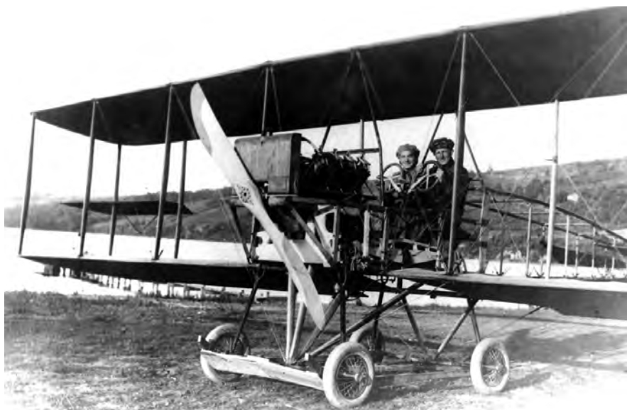
A Curtiss G tractor biplane. First purchased by the Army in 1911, its front-mounted propeller pulled the aircraft through the air.
