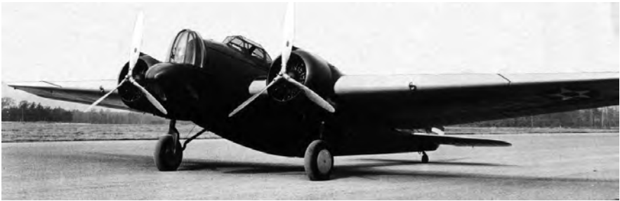
The Martin B-10 bomber featured an enclosed cockpit and retractable landing gear.
