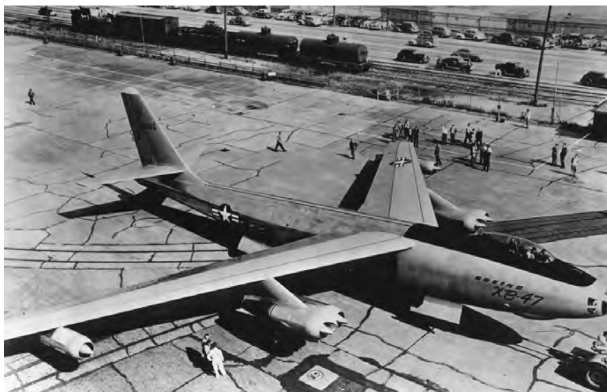
The Boeing XB-47, prototype of the B-47, the first all-jet strategic bomber
