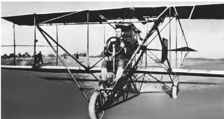
An early Curtiss aircraft equipped with a steering wheel
