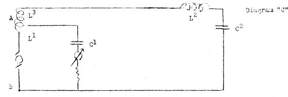
The tube is replaced by an alternator feeding a parallel circuit of low resistance  $L_1C_1$ . The impedence of this is maximum at its resonant frequency. Across this is connected the circuit to be supplied, namely, the antenna, which is a series resonant circuit offering minimum impedence to the frequency to which it is attuned, and by adjusting  $L_2C_2$  so that its period is equal to that of  $L_1C_1$ we have the following ideal conditions.
