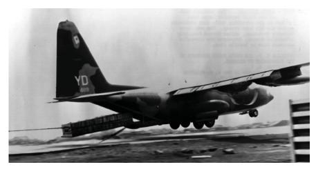
A load of cargo is pulled from an Air Force C–130 at Khe Sanh by a cable attached to the load that has snagged the runway's arrester cable. Using this system, the transport delivered cargo without landing.
