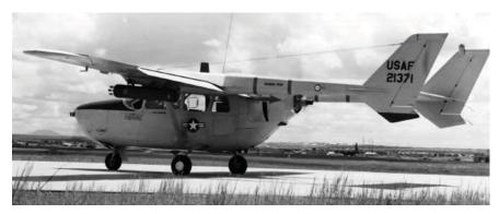
The Cessna O-2 had two engines and hardpoints under the wings.
