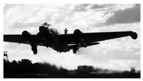
The B–57G, designed for night interdiction, had forward looking radar, low-light TV, infra-red sensors, and a laser range-finder installed in the forward fuselage, but did not perform well in Southeast Asia.
