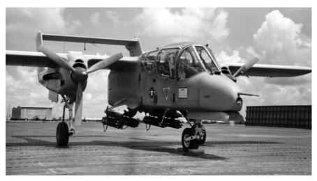
An OV-10 Bronco, with machineguns and rocket pods under the fuselage.
