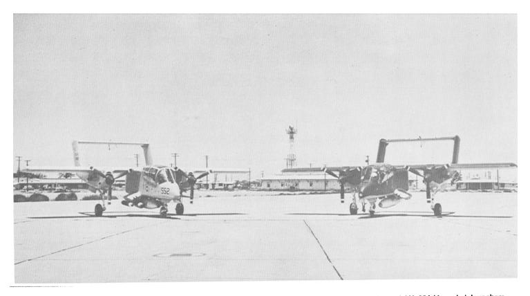
OV-10s shown carrying center line fuel tanks and (on the left) two SUU-11A/A mini-guns and two LAU-32A/A rocket launchers.
