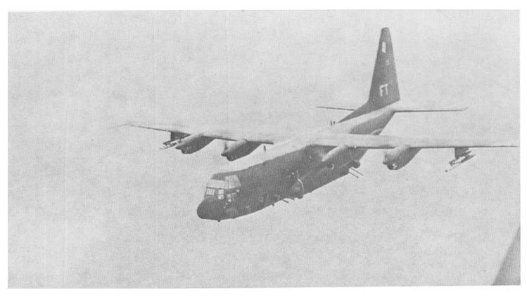
AC-130 "Spectre" Gunship---Note 20mm and 40 mm guns protruding from the side.
