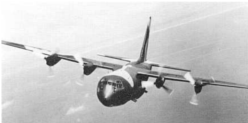
Above: One of the strike aircraft in the Igloo White system was the Air Force AC-130. This gunship received information on possible truck locations while in flight over the Ho Chi Minh Trail. The aircraft commander then attempted to interdict the suspected truck convoys.
